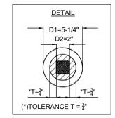
3 WATER VALVE BOX ALIGNMENT DETAIL
