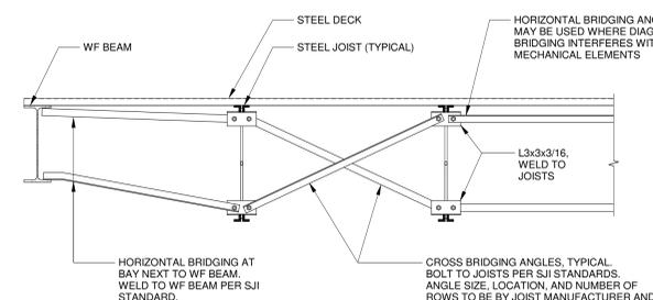
**4 JOIST BRIDGING AT WF BEAM**
