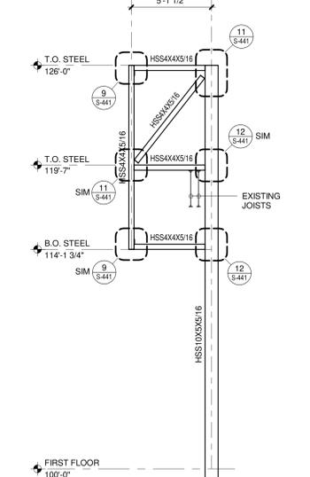
**5 OVERHANG FRAMING ELEVATION**
