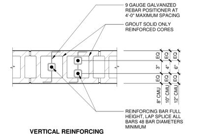
**2 TYPICAL BAR PLACEMENT IN MASONRY CORE**
