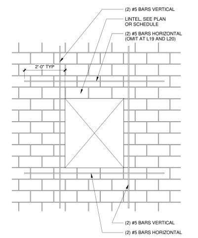
**6 TYPICAL MASONRY OPENING REINFORCEMENT**
