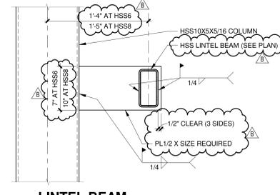
**18 LINTEL BEAM CONNECTIONS TO COLUMN**
