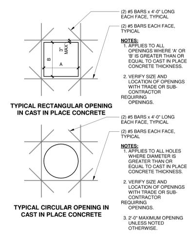
**13 TYPICAL CONCRETE PENETRATION REINFORCEMENT**
