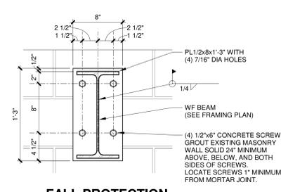
**14 FALL PROTECTION SUPPORT FRAMING AT MASONRY**
