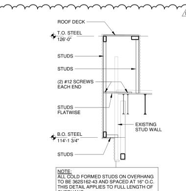
**14 COLD FORMED STEEL FRAMING AT OVERHANG**
