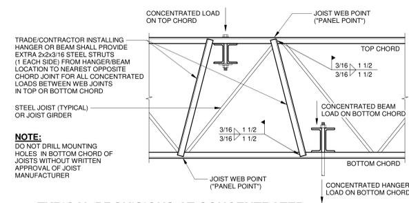
**1 TYPICAL PROVISIONS AT CONCENTRATED LOADS ON OPEN WEB STEEL JOIST/GIRDERS**
