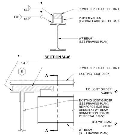
**13 FALL PROTECTION SUPPORT FRAMING AT GIRDER**
