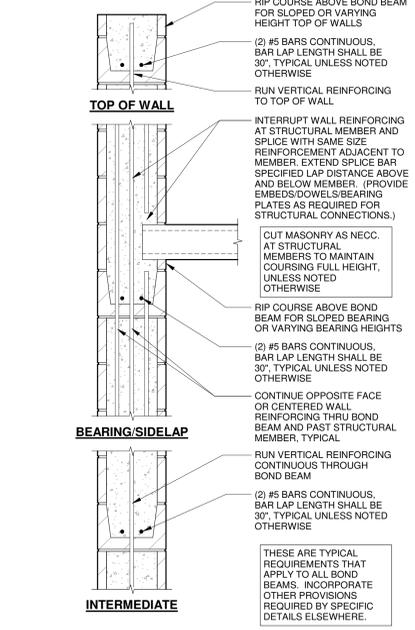
**9 TYPICAL REBAR PLACEMENT IN MASONRY WALL**
