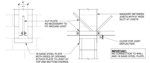
**5 JOIST DEFLECTION PROVISIONS AT NON-LOAD BEARING MASONRY, TYPICAL**
