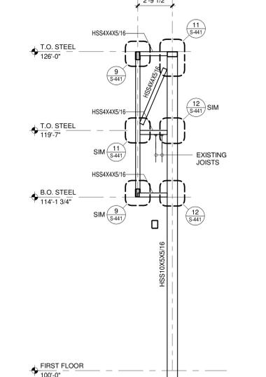
**10 OVERHANG FRAMING ELEVATION**
