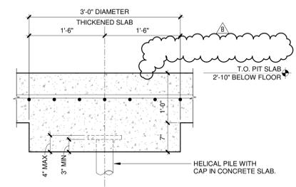
**4 HELICAL PILE AT SLAB - LIFTS**
