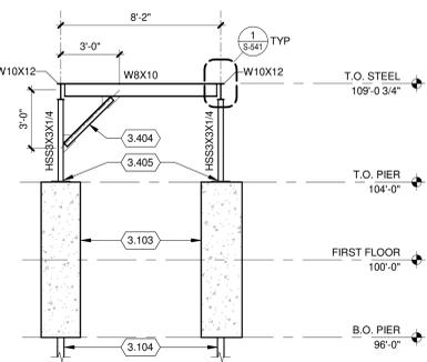
**3 PLATFORM FRAMING ELEVATION**
