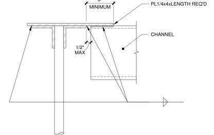
**7 CHANNEL TO JOIST CONNECTION**
