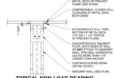
**7 TYPICAL NON-LOAD BEARING MASONRY WALL TOP CONNECTION**
