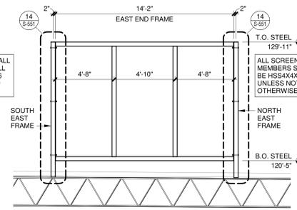
**8 MAU4 SCREEN WALL FRAMING ELEVATION (LOOKING WEST)**
